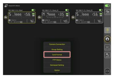
Highlight the slot containing the memory card and tap [**Starts formatting the card...**]. A confirmation dialog will be displayed; tap [**OK**] to format the memory card.
