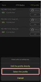
**3.** Tap the (apply) button for the desired FTP profile.
