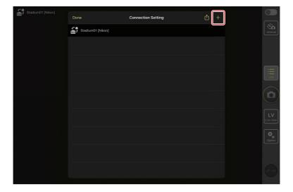
3. Enter the IP address ( 18) and a name for a camera in the remote camera list and tap [Save].
