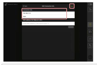
MAC Addresses You need only supply MAC addresses if intend to use the NX Field app's wake-on-LAN feature (C 313) to restart the standby timers on remote cameras.
