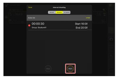
**Taking Pictures Between Intervals** The shutter can be released normally between intervals while interval-timer photography is in progress.
