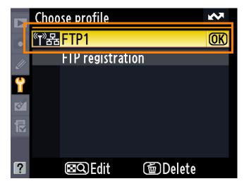
Return to the wireless transmitter menu and turn the WT-4 on. The profile name will be highlighted in green when a connection is established.
